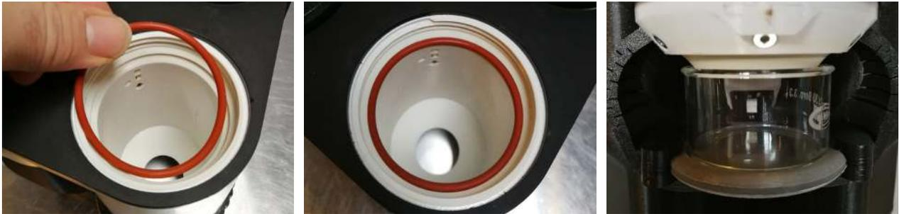
If the gaskets are dirty or greasy from earlier extractions, they need to be cleaned to make an air-tight seal:
