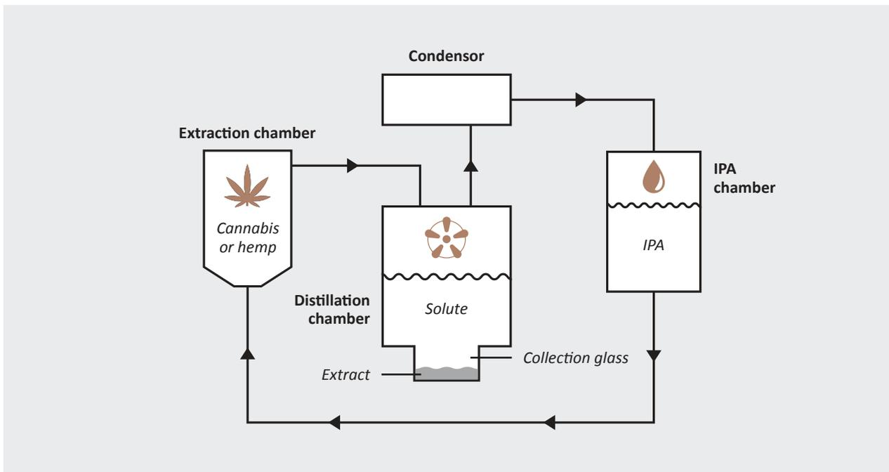
Merlin400 draws the IPA through the herb tube during the extraction, creating a solute (mixture of IPA, cannabinoids, and terpenes). The solute is transferred to the distillation chamber where the IPA is distilled from the solute and recycled as pure IPA back to the IPA chamber.
